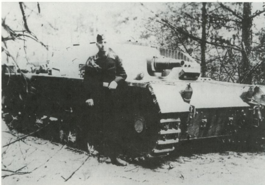
A rare photo of a 's. Pak' from the Veersuchsserie (Experimental Series), which was based on the chassis of the Pz.Kpfw.III Ausf.B. Five such vehicles with soft steel superstructures were built and used for training at the Artillerie Lehr Regiment in Jüterbog. (Chamberlain)
